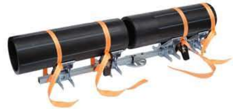
Configuration for "in line" welding
